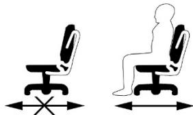
The chair incorporates a safety braking system. When no one is sitting, the wheels lock to prevent the chair from moving accidentally. When someone sits down, they unlock and rotate freely.
