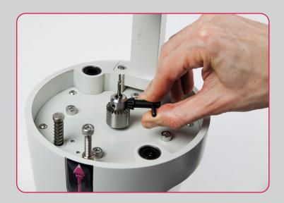
Another significant feature is the smooth operation of the drill. Unlike in some other machines, in the **Atlas** pin drill the table is guided by axial bearings and return springs. The result is astonishing: the touch is firm and accurate, with the exact amount of resistance and elasticity, and without the slightest play. Its smooth sliding, free and without trouble, is difficult to find in other machines of this kind.
