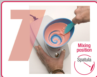
7 After a few seconds, pre-beating is finished. Then, press fast speed (hare) and mix the mixing pressing it with the spatula. The spatula should be placed almost flat against the wall of the bowl. (Mixing position- spatula).
