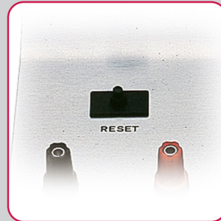
Circuit-breaker with manual reset to prevent overcurrent.
