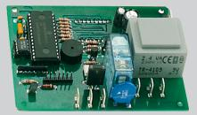
An electronic control is responsible for selecting and executing times. It has acoustic warning signals and a 7-segment digital display.
