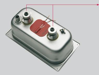
The bath has two powerful sandwich-type transducers with a total power of 100 W transmitted to the tank. Its working frequency (40 kHz) offers an optimal compromise between noise and cleaning power.
