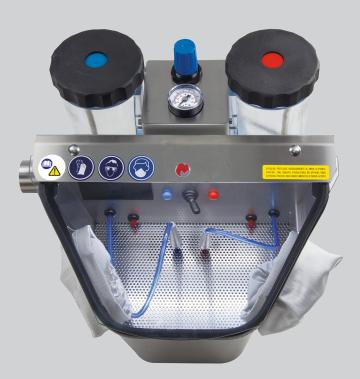
The chamber-change valve is inside the chamber. The colour criterion allows the right chamber to be identified and selected. A rubber attachment inside the chamber may be used for initial adjustments of the sand jet.
