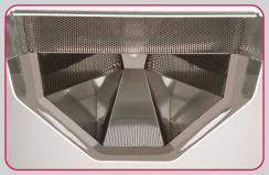
The sand hopper deposit has a capacity of 12 Kg. Its volume, along with its great depth and its steep walls, allows to operate the machine in full automatic mode for more than 30 minutes.
