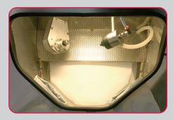
The sand in the hopper deposit is absorbed by the Venturi aspiration and then it is pressure-injected by the nozzle. Then it falls again into the hopper deposit.
