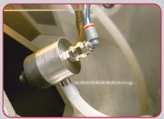
The sand flow moves along a closed circuit pushed by a Venturi-type pneumatic system.
