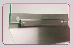
The glass has a special protection shield. This surface reduces the abrasion effect of the sandblast and prevents accidents, should the glass break. The glass is very easily replaced.
