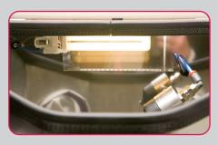
The lighting is made through a powerful fluorescent lamp that offers a good chromatic reproduction without brightness. A transparent polycarbonate screen protects the lamp from sand blasts.
