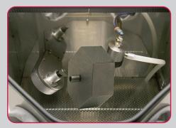
The basket can be easily disengaged from the motor shaft, which makes preparing the works easier.
