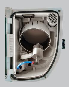
The basket can be easily uncoupled from the drive shaft, which simplifies the preparation of the works.
