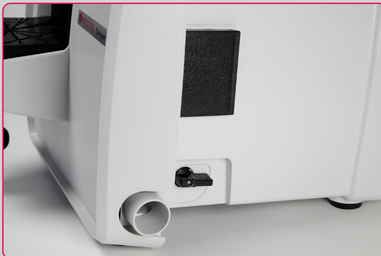
Water-inlet tap and lateral water outlet.
