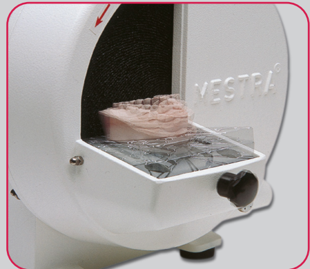
Easy-to-extract, 3-position, fold-down table (80, 90 & 100°). Marked for referencing trimming on precision models.
