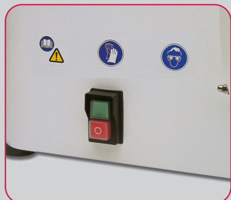
Safety switch: if electricity fails the unit is disconnected and must be manually reset (thus preventing accidental start-up).
