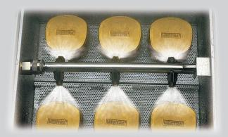
The washing system with 6 highpressure water injectors ensures proper scalding of flasks and perfect wax removal.
