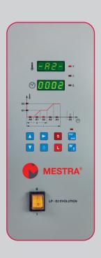
Twin display screen: one for temperature, the other for time.
