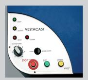
The control panel is synoptic, allowing easy handling. Three control buttons and a potentiometer to regulate melting are sufficient to carry out casting. The melting point can even reach 1750 °C. The state of the process is visualised by four pilot lights.
