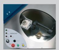
Access to the interior is wide thanks to the large upper window. The arm of the Vestacast is self-expanding with return springs, which means that maximum centrifuge acceleration can be achieved when the machine starts up. The lightness of the arm considerably reduces the vibration commonly found in this kind of apparatus.
