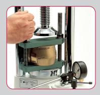
The width between columns and the diameter of the top plate enable flasks to be put in and taken out with the MESTRA Ref. 030380-90-400-410 clamps for press with no need to raise the spindle. This saves time and trouble.
