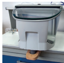
Docking coupling with Jeb type suction.
