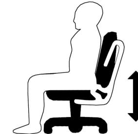
Sit down, press the handle up and let the seat go up to the desired height. Down the handle again to fix the height.
