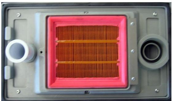
3. Place the new cartridge filter, and proceed to assemble the rest of the components.
