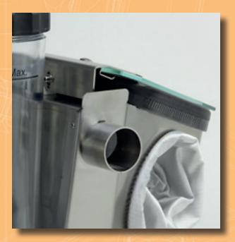
Dust exits the chamber via a tube at the side of the machine, to which any conventional suction unit may be connected, ready for work with silicon oxide. MESTRA recommends references R-080532 Eolo plus and R-080539 Gemini.
